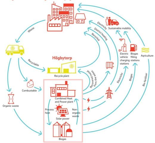
Electricity, heating and biogas from rejected residual products
