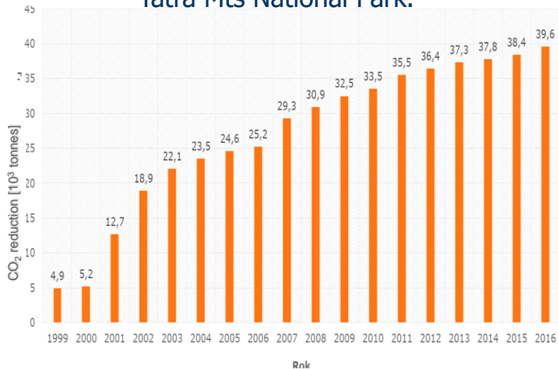
Zakopane: CO 2 reduction thanks to geoDH (since 2001). Source: PEC Geotermia Podhalańska S.A.)
